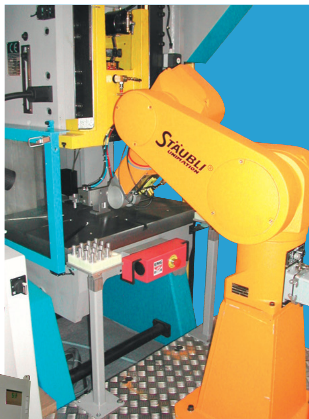
25 T press with automatic robotic loading
