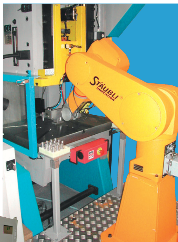
25 T press with automatic robotic loading
