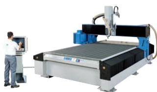
MECAPLUS High productivity 3 axis CNC milling machine
