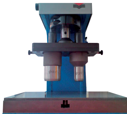
Pneumatic press with electric controlling cabinet.
