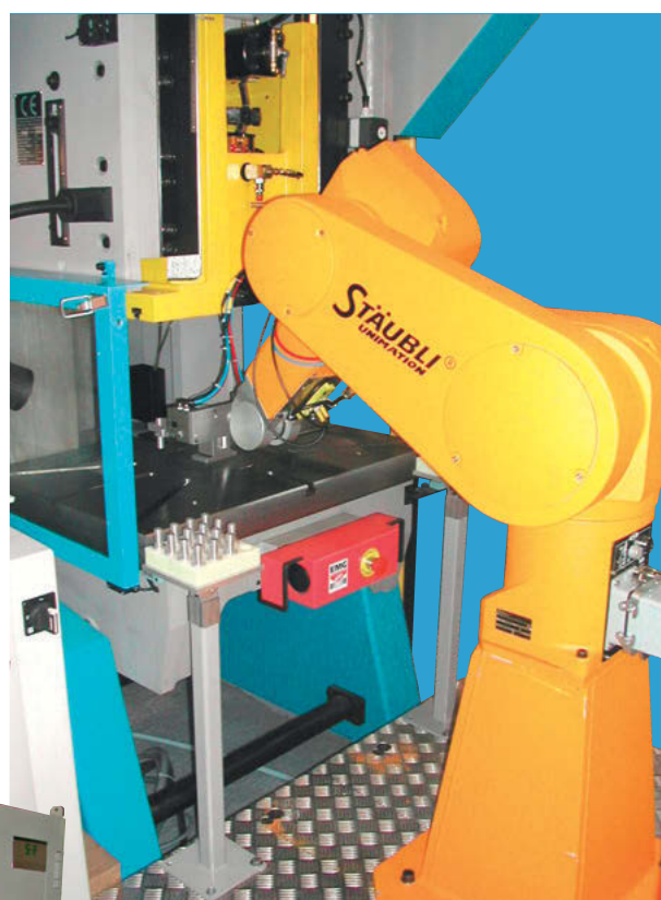
25 T press with automatic robotic loading
