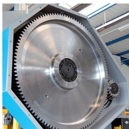
View of the 80T sprocket pinion assembly
