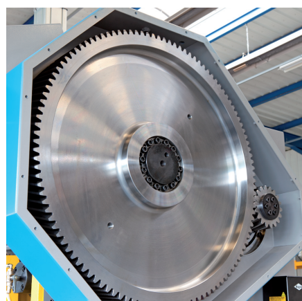
View of the 80T sprocket pinion assembly
