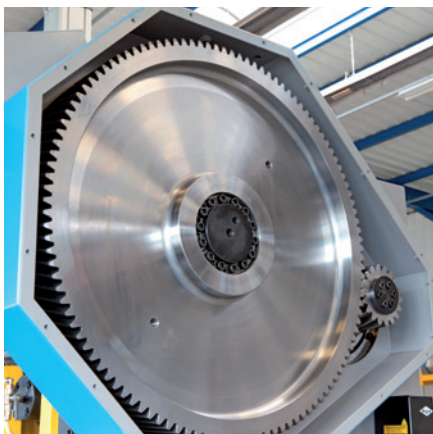
View of the 80T sprocket pinion assembly
