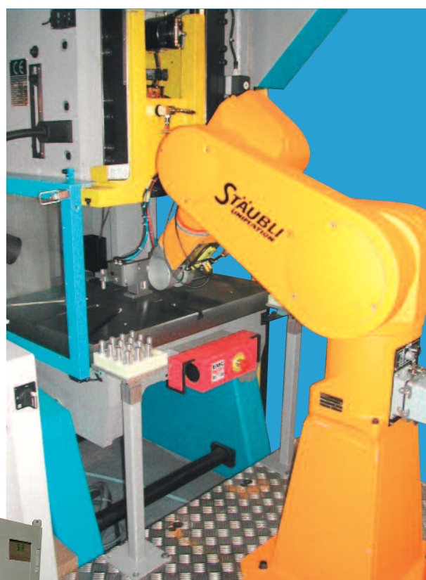
25 T press with automatic robotic loading
